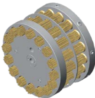
Diagram of a deburring device for deburring end brushes
