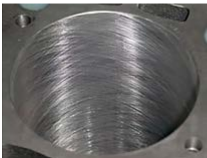
Example of the cross-hatch finish achieved by honing.
