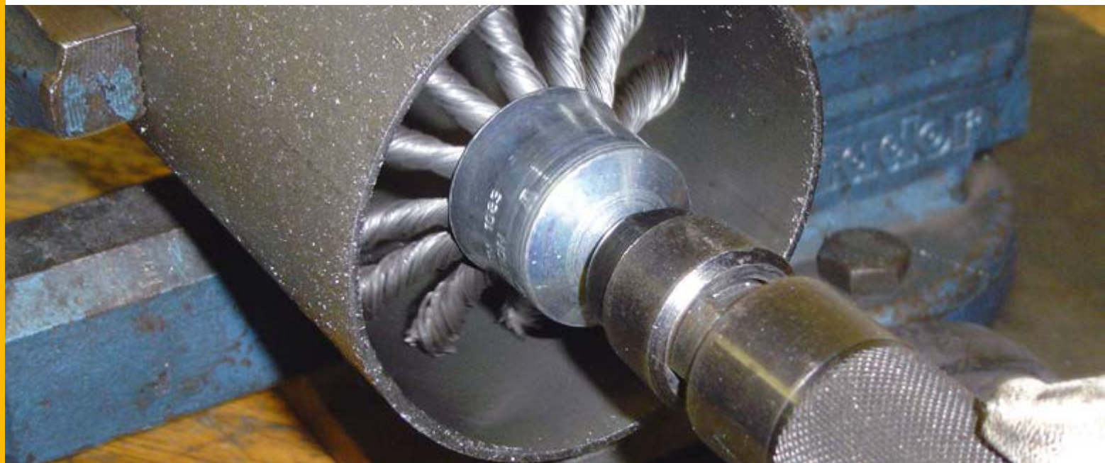
Opening of end brushes as a function of speed
