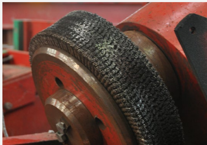
Multiple individual rings make a powerful brush
