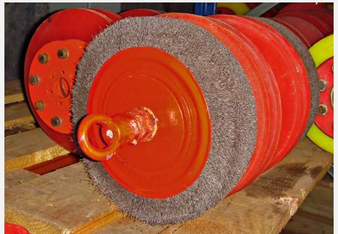
A cleaning pig with several installed roller brushes
