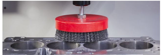
Deburring a motor block with a disc brush (wire brush filling material)
