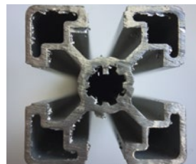
Component before deburring
