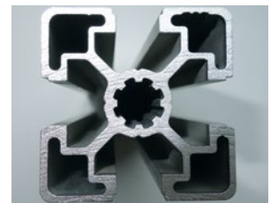
Component after deburring
