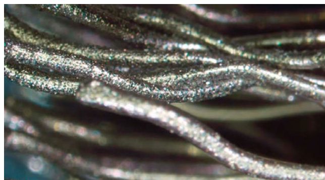
The picture shows diamond brush filling material. Diamond brush filling material is particularly suitable for aggressive applications and for materials with high material strength.
