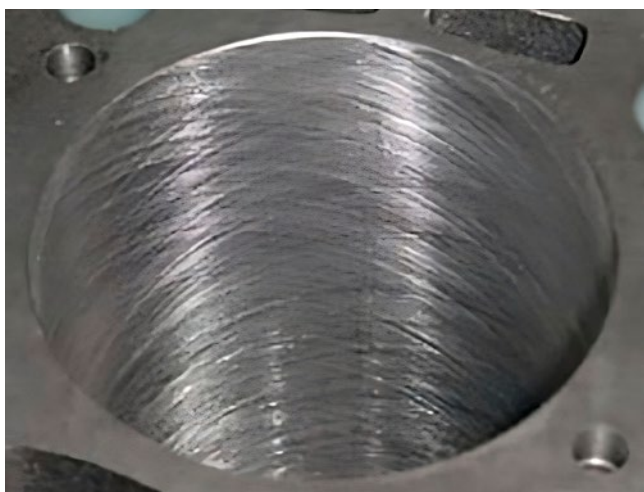
Example of the cross cut produced during honing
