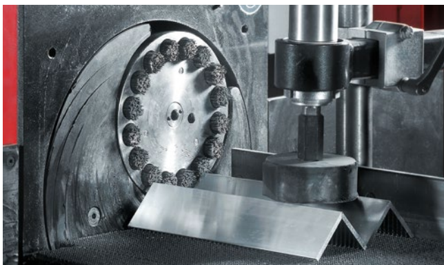
Application of deburring end brushes
