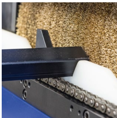
Function chart of a deburring machine with roller brushes
