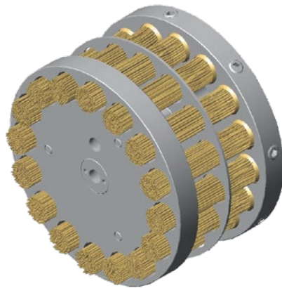
Schematic diagram of a deburring device for deburring end brushes
